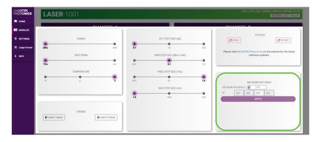
The value in the 3<sup>rd</sup> octet of the IP address can be changed to any available value. It is important to make sure that any other instruments connected to the computer do not share this new IP address, as there will be an addressing conflict.
