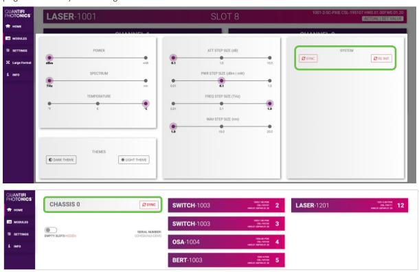
Clicking the **RE-INIT** button will bring up a prompt to continue, since this action will temporarily disconnect all modules while the re-initialization with the CohesionDriver service is in progress. Once it is complete, the page will be functional again.
