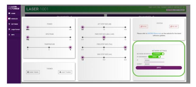
The addressing method can be changed to a static method, where the MATRIQ instrument will always have the same IP address over Ethernet. Typing in a **valid IP address and Subnet mask**, and then clicking **APPLY** will save the IP address into the settings of the instrument.
