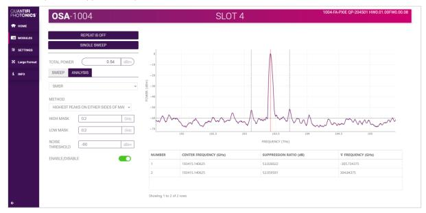
A non-symmetric mask can also be applied with this SMSR method, to facilitate SMSR calculation between other side modes. In the example below, the SMSR is calculated between the peaks at approximately 193.109 THz and 194.030 THz.
