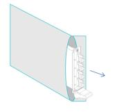
STEP 5: Engage the fastening clip. Secure all fastening screws
