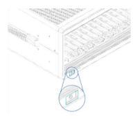
STEP 2: Remove the module from the antistatic bag. Retain bag
