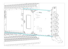
4 Push module into slot until you feel resistance from the backplane connection.
