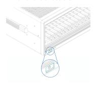
2 Unsecure the fastening screws and fastening clip.
