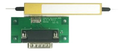
The IQABC adaptor board comes in either single polarization or dual polarization versions to match your IQ modulator. If your modulator is not OIF compliant, you can use the IQABC's custom break-out cable instead of the adaptor boards, which can be purchased separately.
