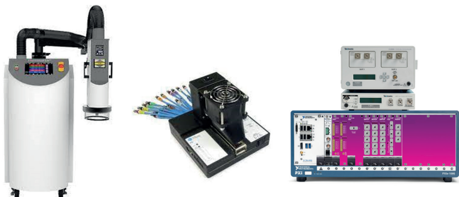
Image 15: Key equipment for module test - thermal stream, MSA-compliant MCB, test instrumentation.
