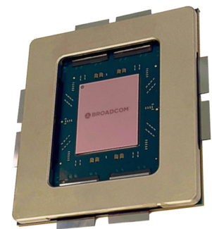
Image 5: A Broadcom Co-Packaged Optical device (Source: Broadcom).
