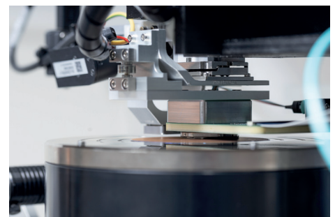
Image 22: Multiple device e/o test head over VCSEL wafer ( Source: ficonTEC)
