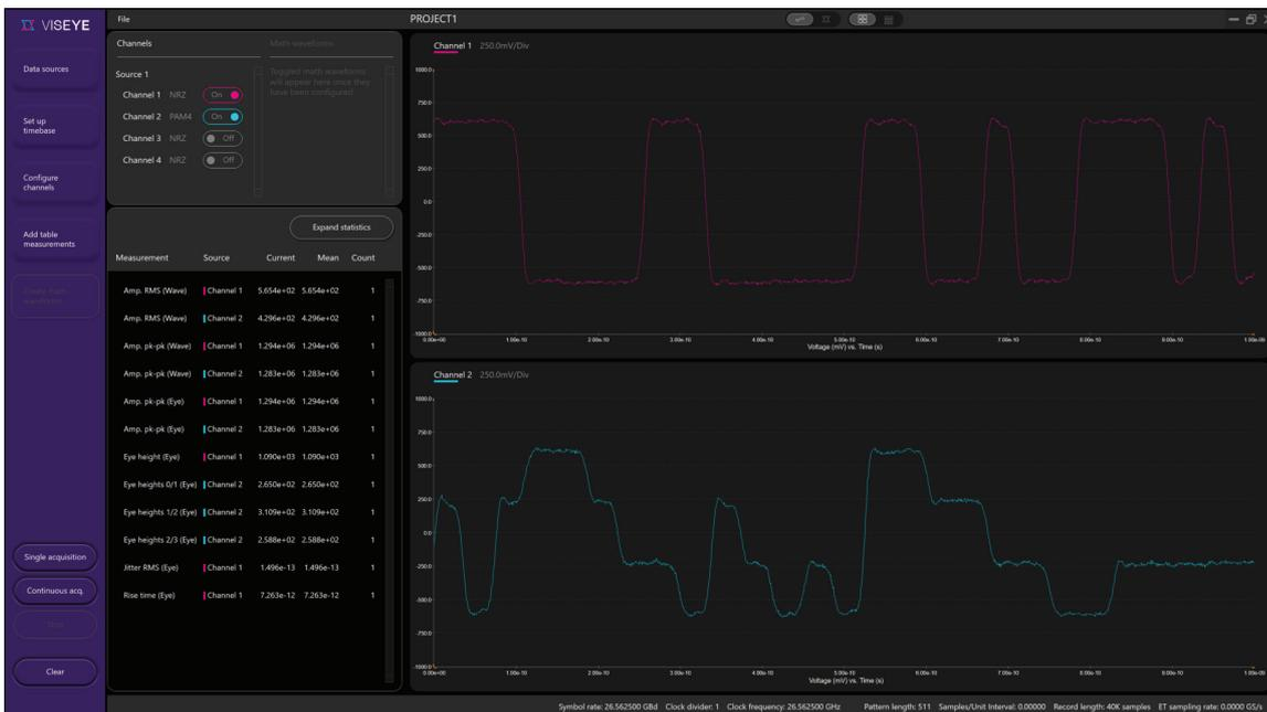
Image: 26 GBaud PAM4 trace plot shown with statistics of the numerical parameters.
